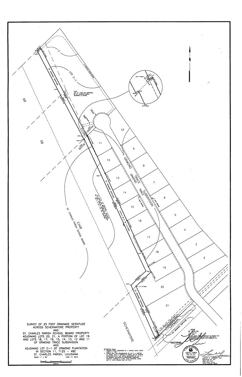
distance of 595.37 feet, thence N45°36'23"E a distance of 26.12 feet, thence S27°32'14"E a distance of 595.38 feet, thence N45°37'14"E a distance of 2.79 feet, thence S24°55'06"E a distance of 897.43 feet, thence S46°26'12"W a distance of 123.41 feet, thence S24°55'06"E a distance of 318.23 feet to the point of beginning, containing 48,354.37 square feet or 1.110 acres all in accordance with a plan by Lucien C. Gassen, PLS, dated June 17, 2015 attached hereto and made a part hereof.
