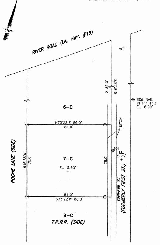
NOTE: THE FRONT CORNERS WERE SET ON A 5' INSET DUE TO THE PROPERTY LINE FALLING IN THE DITCH
