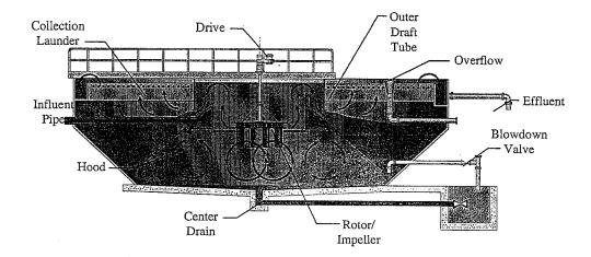
The slurry is in controlled motion, outward and downward. From it the treated water is displaced upward. The slurry is drawn back under the hood structure to the primary mixing and reaction zone by the suction produced by the impeller. Recirculation of the slurry is independent of the flow rate. Because of this unique feature, rapid changes in flow rate can be handled.
